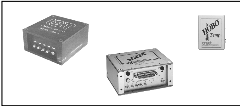
Figure 3 Examples of self-contained electronic field data recorders
